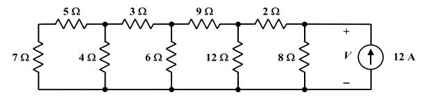
a. Using series and parallel resistance reductions, find the equivalent resistance seen by the source.
